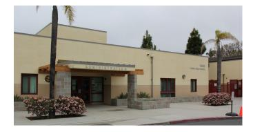
Torrey Hills School was constructed in 2002. It includes multiple plaster skinned, single story buildings with steel-framed covered walkways, eight Modular classrooms, a Multi Use Room (MUR), and a Library Building. Roofing is a combination of flat and sloped roofs.
